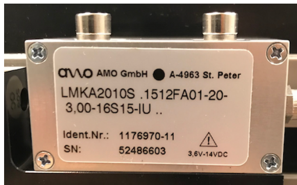
Figure 6. The correct full-gap encoder readhead model (LMKA-2010S.1512FA01-20- 3,00-16S15-IU).
