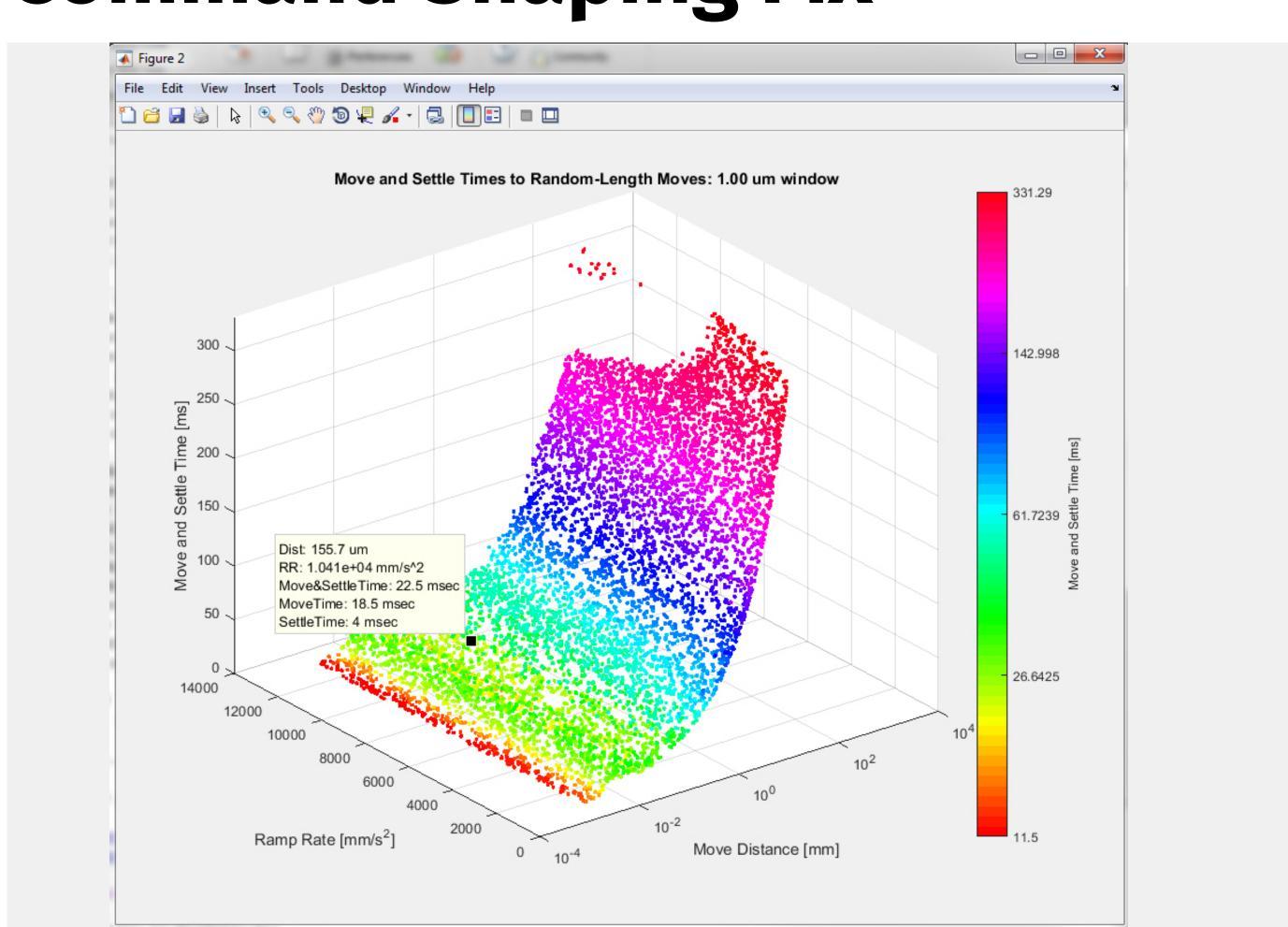
After finding the frequency that caused the anomaly we were able to use command shaping to remove the frequency component from the acceleration command, which removes the excitation that caused this anomaly.
