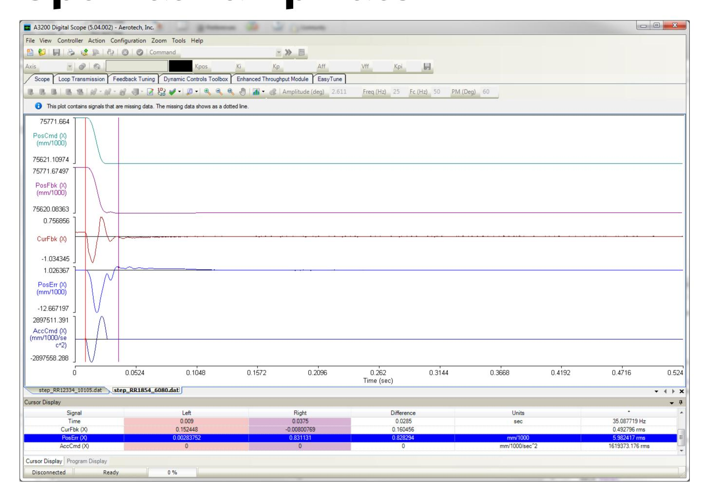
An optimal ramp rate does not show this oscillation.
