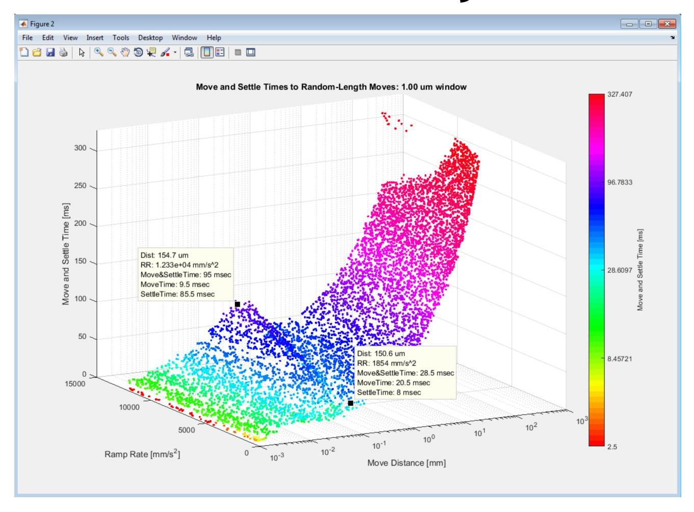
Took a bunch of plots of random move distances and acceleration rates. The dip in the middle showed an anomaly in the move profile caused by the base of the stage.
