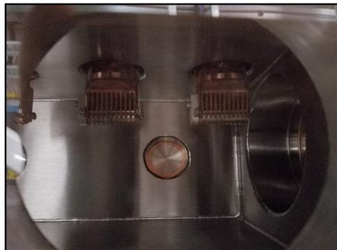
Figure 2: Motor-driven Beryllium lens arrays used to focus the LCLS X-rays located inside the Transfocator.
