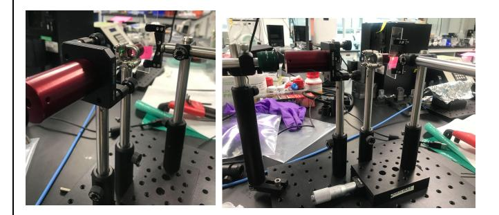
Encountered difficulty with aligning collimator and smaller size focusing assemblies, printed adapter to join
