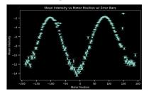
The data was fitted with a sine squared curve to the graph, and then extracted the maximum and minimum values with the maximum corresponding to  $I_{0^{\circ}}$  and the minimum corresponding to  $I_{90^{\circ}}$ , in the following equation. This was done using the Python package Imfit.
