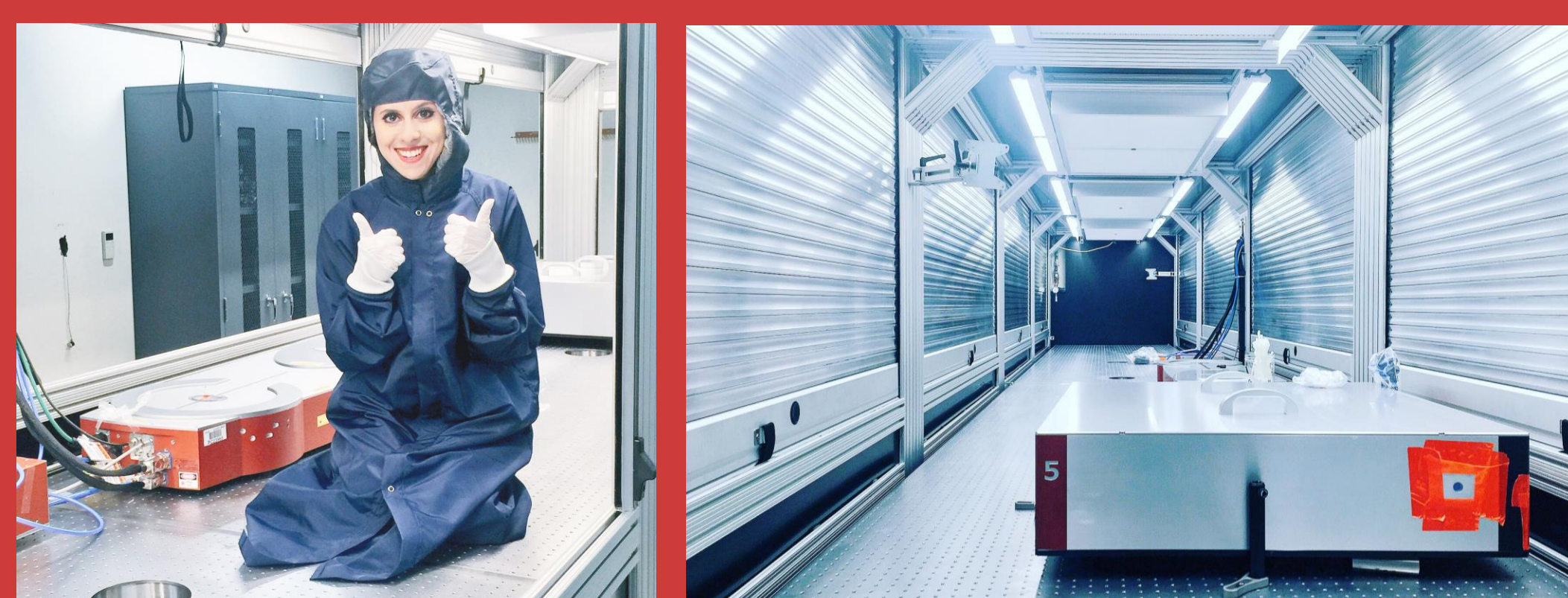
Figure 1: Top left and right: laser enclosure for IGNIS. Bottom left: cleaning the inside of the laser enclosure so that optics are not damaged when the laser is on. Bottom right: inside of laser enclosure.
