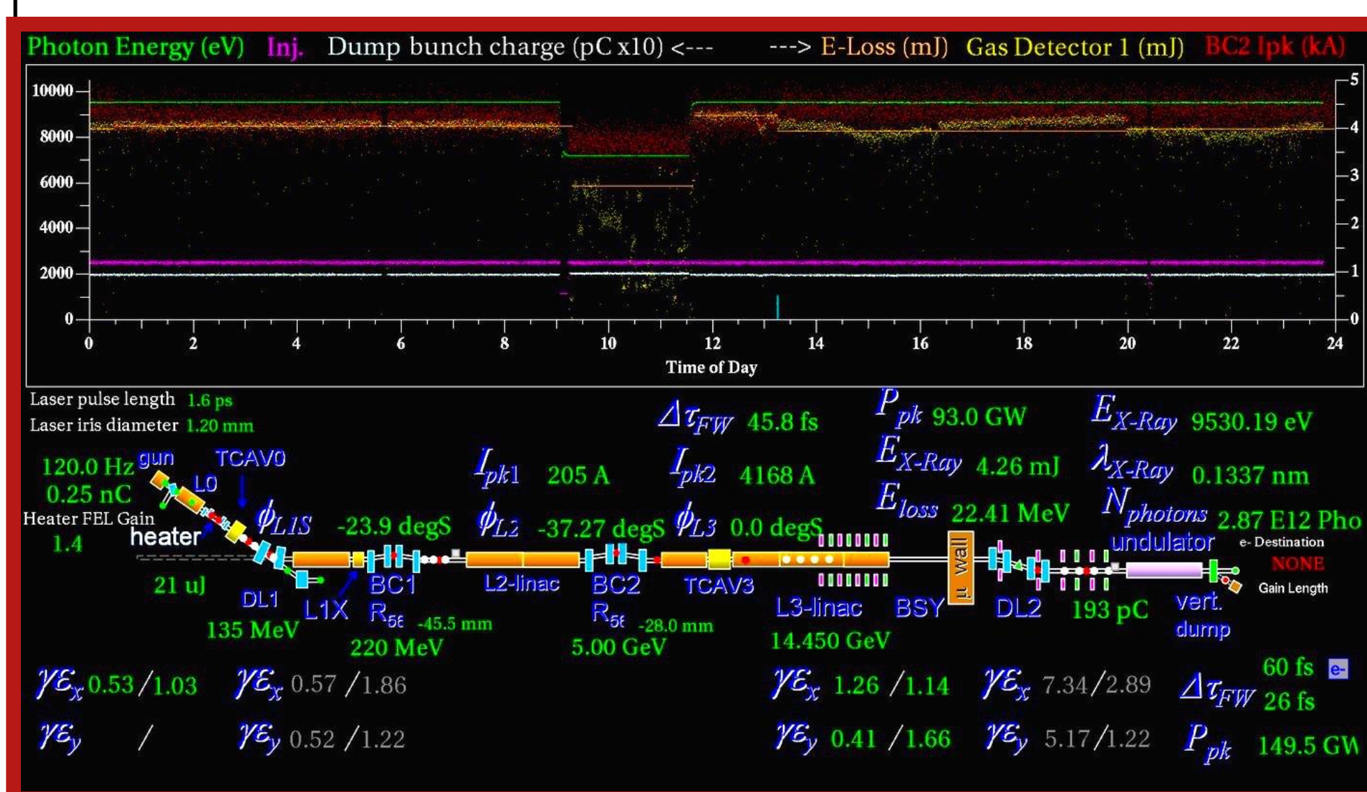
Figure 1: A screenshot of the control room LCLS summary display. Here, one can see how the FEL performs when certain parameters are varied.
