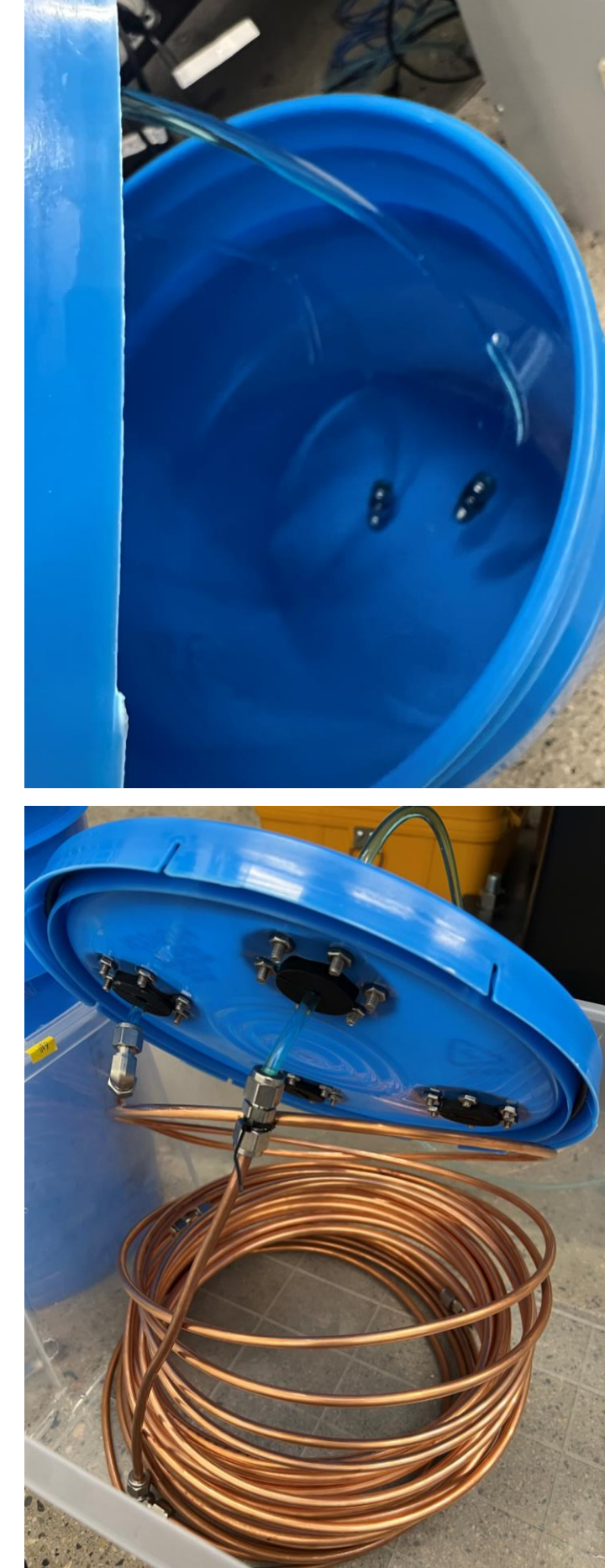
Fig 4: Open lines pour in the bucket (Top) Fig 5: Closed copper coil loop (Bottom)
