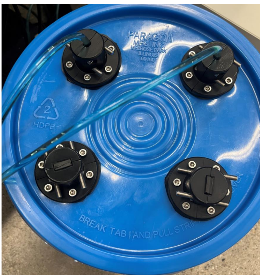
Fig 2: Bucket lid with feedthroughs installed (Right) Fig 3: CAD model of clamshell waterline feedthrough (Left)
