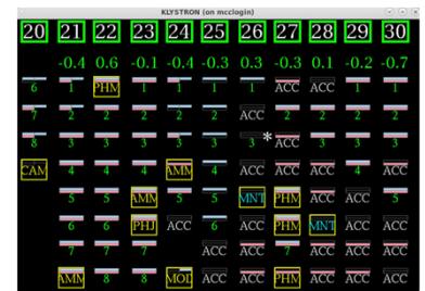
Fig 7. EDM "mini" klystron display, updated for dual energies. Pink bars correspond to the SXR beamline, and blue bars to the HXR beamline.
