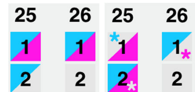
Fig 4, 5. A subset of the klystron complement, displayed with "Show diff" toggle off (left) vs. on (right). Blue color = klystron on beamcode 1 Pink color = klystron on beamcode 2
