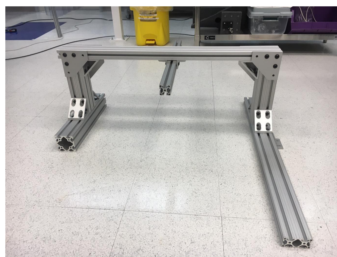
Fig 4. Top View of Gantry Mount. Camera and autocollimator will be mounted.
