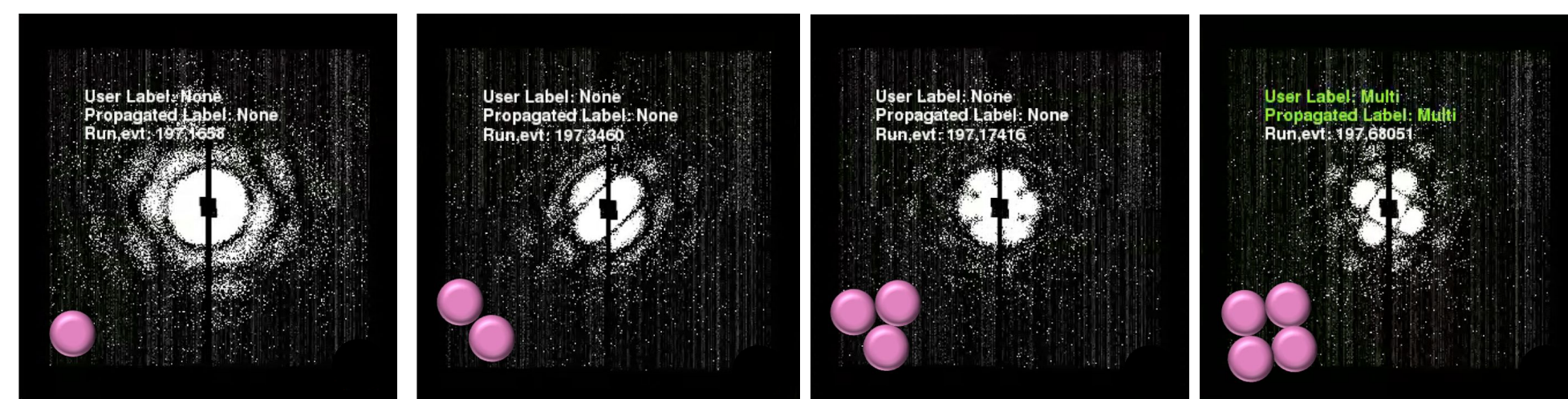
Figure 1: Diffraction from single, double, triple, and quadruple PR772 virus hits at LCLS.
