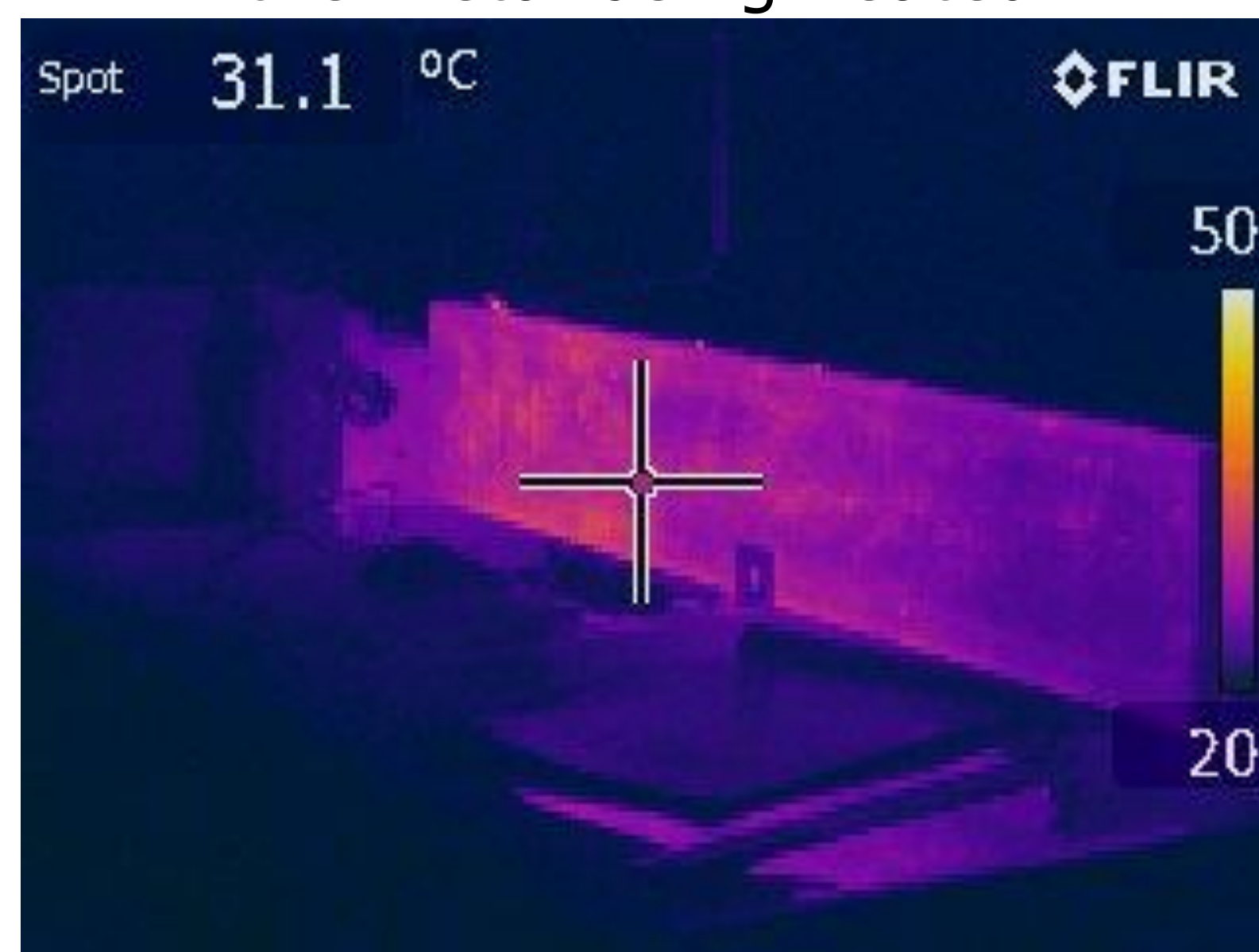
Fig E: Steel with no wrap
