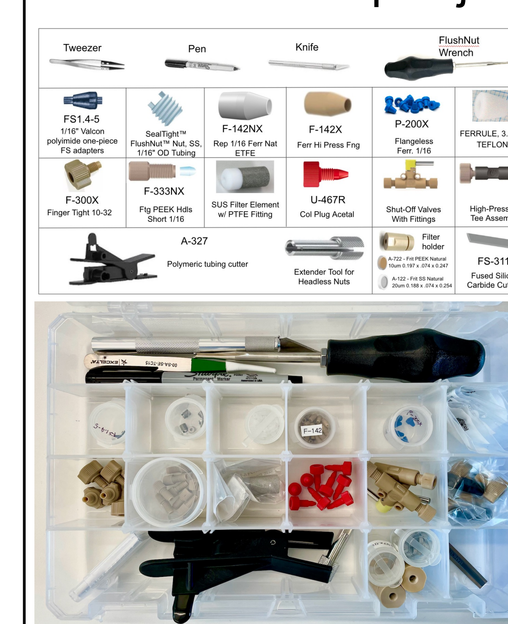
Fig 7. A list of the toolbox and a picture of the toolbox. It includes essential parts in setting up the liquid jet, such as adaptors, ferrules, filters, valves, cutters, wrenches, tweezers, etc.
