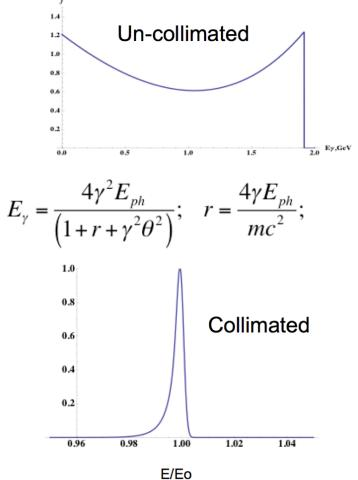
High-energy beam combined with state of the art laser systems deliver unprecedented combination of gamma-ray energy and flux
