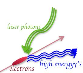
Polarized gamma beams 2 MeV - 4 GeV with high flux  $10^{9}$ - $10^{11}$  γ/sec for diverse research programs
