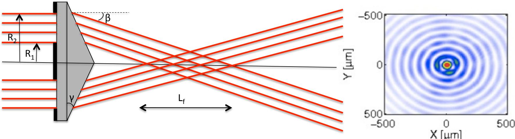
The depth of focus  $L_f$  is given based on the geometry consideration as:
