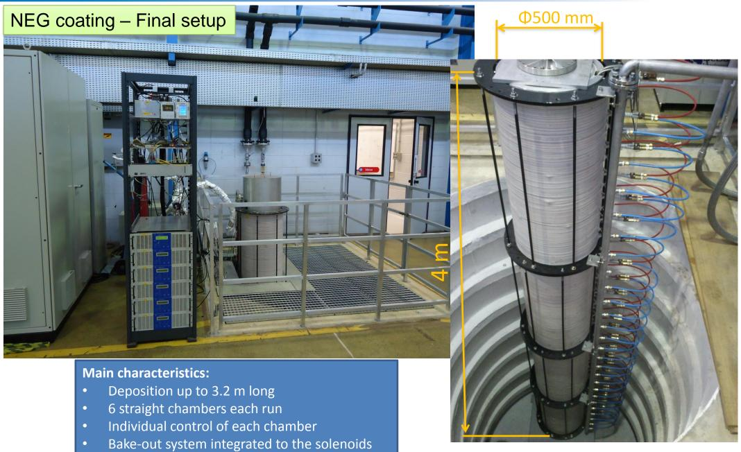
• Automatic control of the whole deposition run
