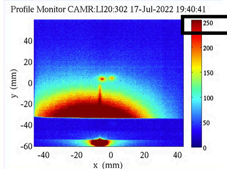
Gamma signal after 10 min at 10Hz
