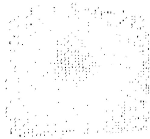
Fig. 7. 15 GeV/c \pi^- incident on a 4.2 mm Ge single crystal. Same plot and condition as in fig. 6. Here planar effects are absent but there is a peak in the axial direction surrounded by a low-intensity region. Note that the axial peak is lower than the random "plateau" far from the axis. There are 10 000 events in the plot.
